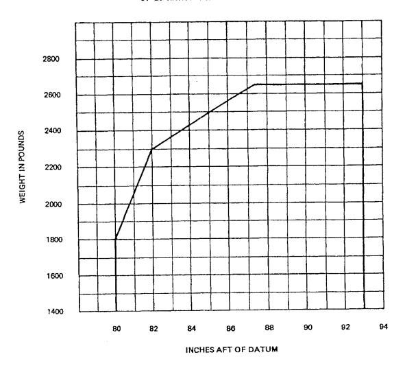
MOMENT DUE TO RETRACTING LANDING GEAR = +819 IN - LBS
