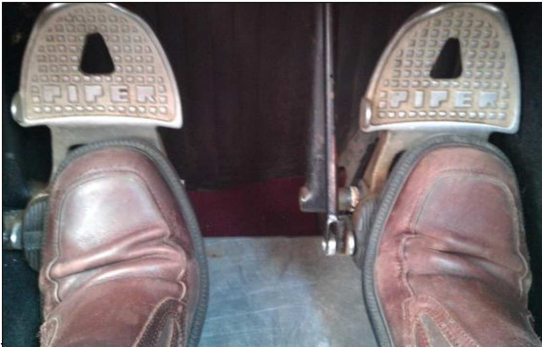
Figure 1: Proper feet position on the rudder pedals and not on brakes
